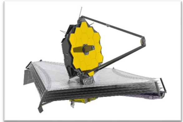
Figure 2: The JWST's sunshield is as big as a tennis court. Credit: European Space Agency/ATG medialab
